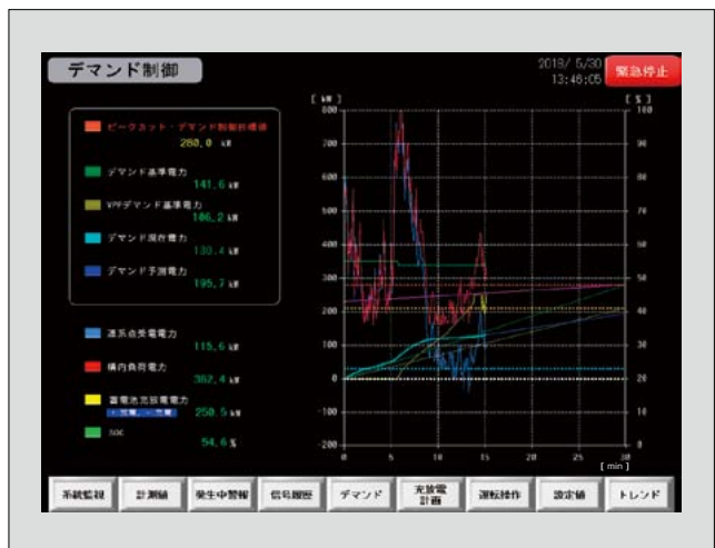
Fig.8 Example of demand monitoring screen
