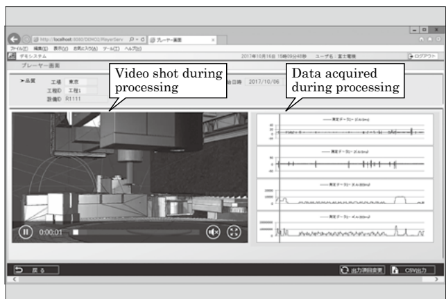
Fig.3 Sample screen of camera-server linking function
