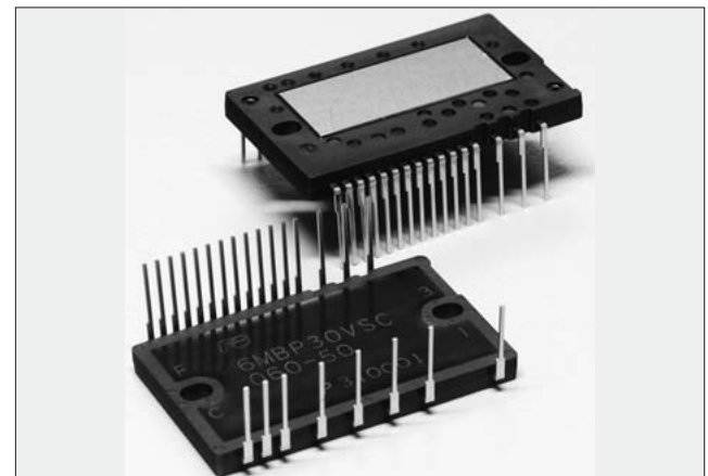
Fig.2 Small IPM for industrial use
