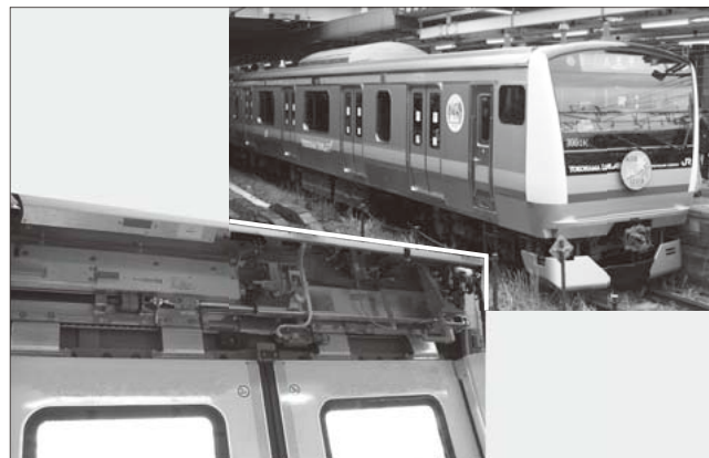
Fig.11 E233 series vehicles for Saikyo Line and Yokohama Line and linear door system
