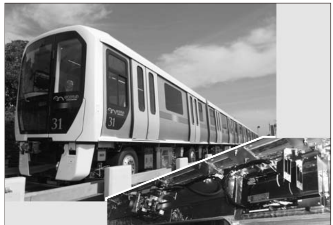
Fig.9 Yurikamome 7300 series vehicle and door system
