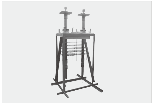
Fig.10 Temperature variable current lead
