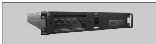
Fig.6 Step-down transformer box
