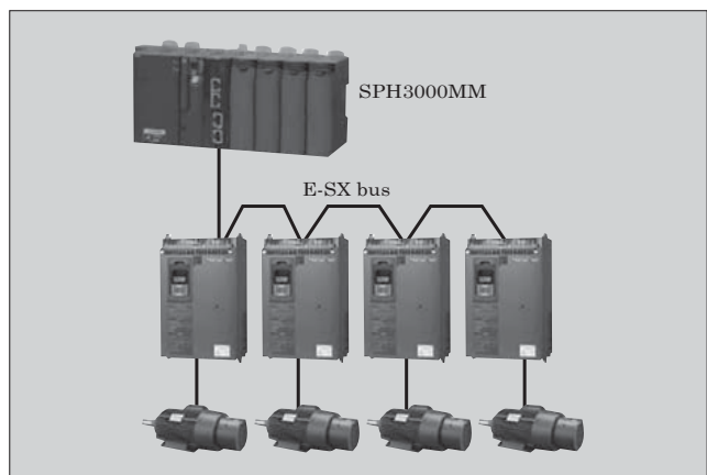
Fig.5 System configuration of E-SX bus
