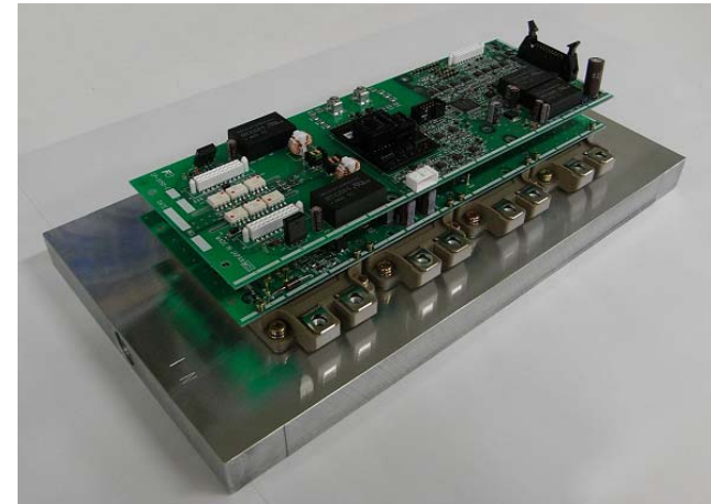
Water cooled inverters
