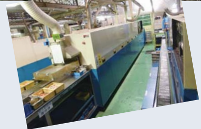
Components laid out on a carbon tray (top), welding in a high-temperature furnace
