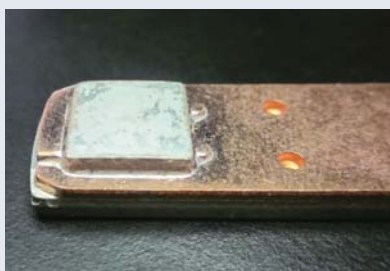
The silver has melted adequately during welding, thereby firmly welding the two components together. Yields are up thanks to on-site initiatives.
